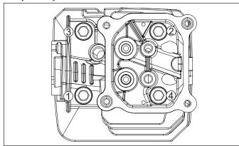
NOTE: Do not reuse cylinder head screws or gasket. Always replace with new screws or gasket.
