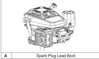
NOTE: Pull on boot only, to prevent damage to spark plug lead.
