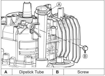
Insert dipstick tube into oil pan and secure to crankcase with screw. Torque screw to 8  $N\!\cdot\!m$  (71 in. lb.).
