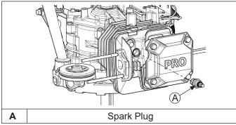
Remove spark plug from cylinder head.
