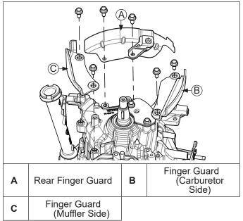
Remove screws and finger guards from crankcase.
