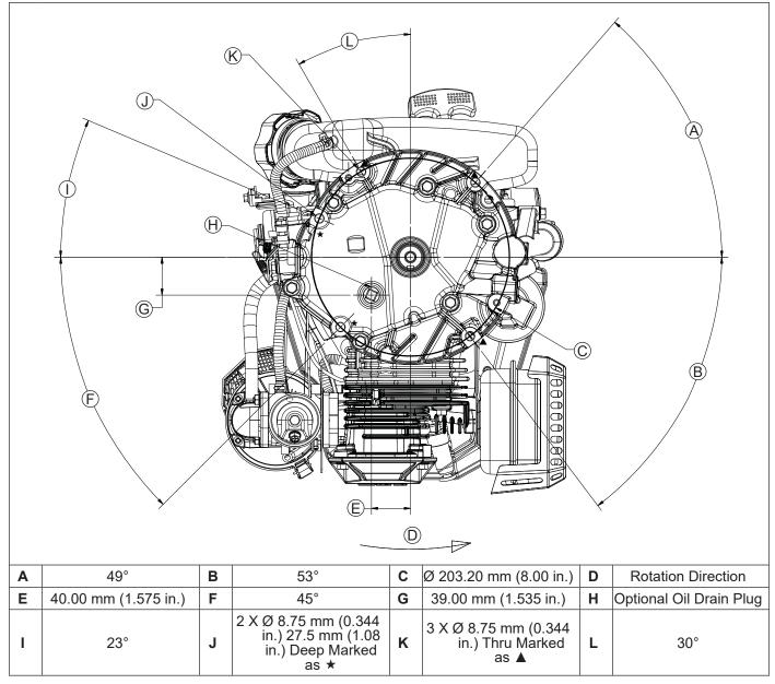
CV200, CV224 Engine Dimensions-Flywheel Side
