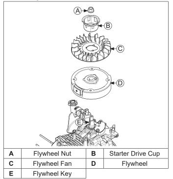
1. Using a flywheel strap wrench to hold flywheel, remove nut inside drive cup.
