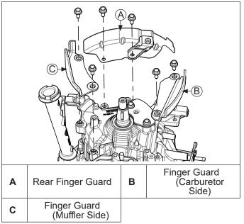
Install finger guards and secure with screws. Torque side guard screws to  $9.5 \text{ N} \cdot \text{m}$  (84 in. lb.). Torque rear guard screws to  $10 \text{ N} \cdot \text{m}$  (89 in. lb.).
