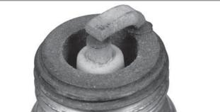
Plug taken from an engine operating under normal conditions will have light tan or gray colored deposits. If center electrode is not worn, plug can be set to proper gap and reused.
