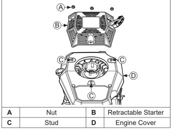
Remove nuts securing retractable starter assembly to engine cover; lift starter off studs.
