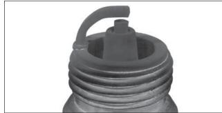
Soft, sooty, black deposits indicate incomplete combustion caused by a restricted air cleaner, over rich carburetion, weak ignition, or poor compression.
