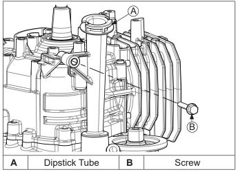
Remove screw securing dipstick tube to crankcase; remove tube.
