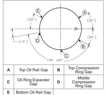
NOTE: Rings must be installed correctly. Install oil control ring assembly (bottom groove) first, middle compression ring (center groove) second, and top compression ring (top groove) last. Oil control ring assembly is a three-piece design, and consists of a top rail, expander ring, and bottom rail.
