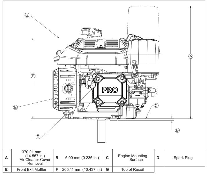
CV173 Engine Dimensions-Fuel Tank Side
