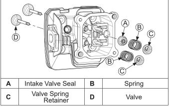
NOTE: Only intake valve has a seal. There is no valve seal on exhaust side.
