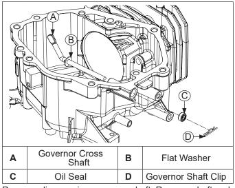
Remove clip securing governor shaft. Remove shaft and washer.
