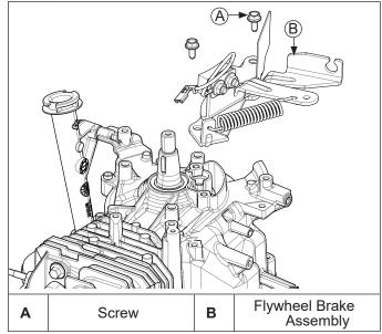
Remove screws and flywheel brake assembly from crankcase.
