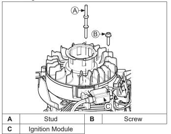
NOTE: Ignition kill lead can stay connected to ignition module.
