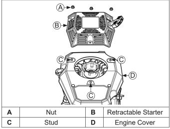
Place retractable starter onto studs and secure with nuts. Torque to 8 N  $\cdot$  m (71 in. lb.).
