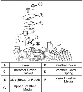
Breather system is designed to control amount of oil in head area and still maintain necessary vacuum in crankcase.
