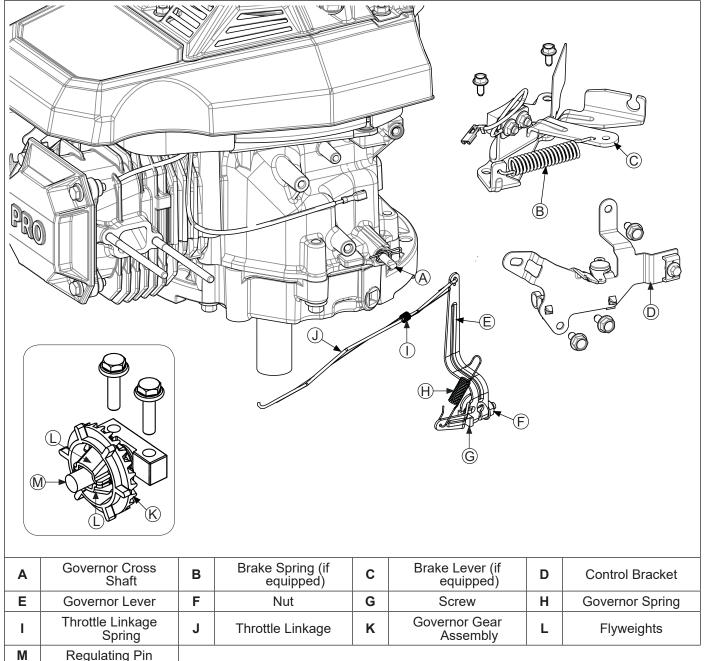
Governed speed setting is determined by position of throttle control. It can be variable or constant, depending on engine application.
