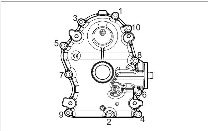
RTV sealant is used as a gasket between oil pan and crankcase. Refer to Tools and Aids for a listing of approved sealants. Always use fresh sealant. Using outdated sealant can result in leakage.
