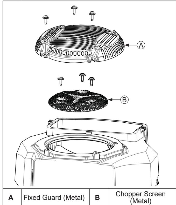
1. Remove screws securing metal guard to blower housing. Remove guard.
