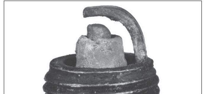
On a worn plug, center electrode will be rounded and gap will be greater than specified gap. Replace a worn spark plug immediately.
