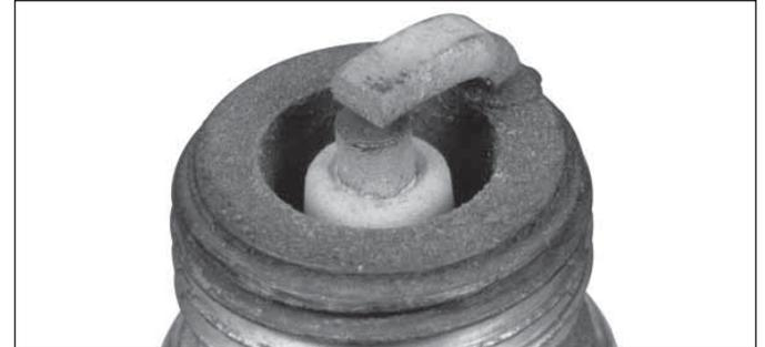
Plug taken from an engine operating under normal conditions will have light tan or gray colored deposits. If center electrode is not worn, plug can be set to proper gap and reused.
