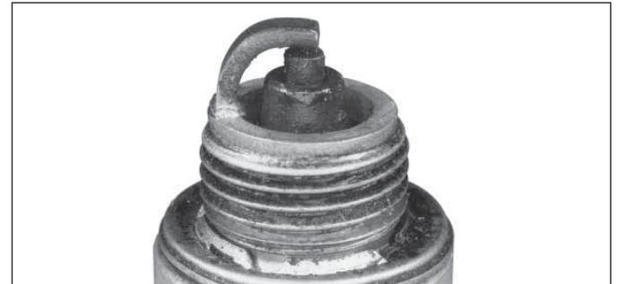
A wet plug is caused by excess fuel or oil in combustion chamber. Excess fuel could be caused by a restricted air cleaner, a carburetor problem, or operating engine with too much choke. Oil in combustion chamber is usually caused by a restricted air cleaner, a breather problem, worn piston rings, or valve guides.
