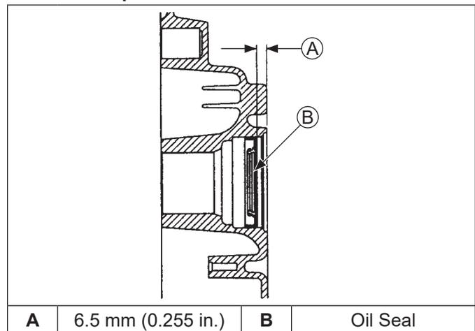
1. Check to make sure there are no nicks or burrs in crankshaft bore of oil pan.
