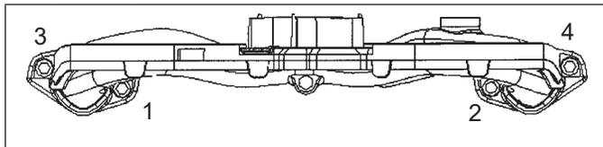
1. Install intake manifold using new O-rings, with wiring harness attached, onto cylinder heads. Slide any wiring harness clips onto appropriate bolts before installing. Using sequence shown, torque screws in 2 increments, first to 7.4 N·m (66 in. lb.), then to 9.9 N·m (88 in. lb.).
