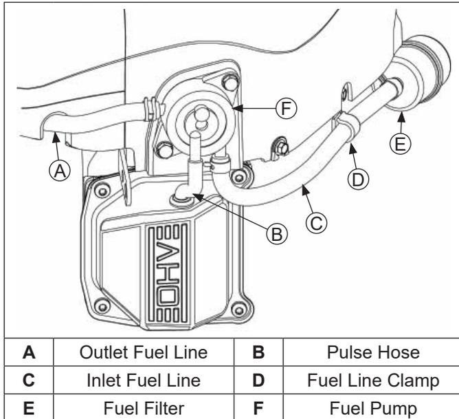
NOTE: If a new fuel pump is being installed, make sure orientation of new pump is consistent with removed pump. Internal damage may occur if installed incorrectly.
