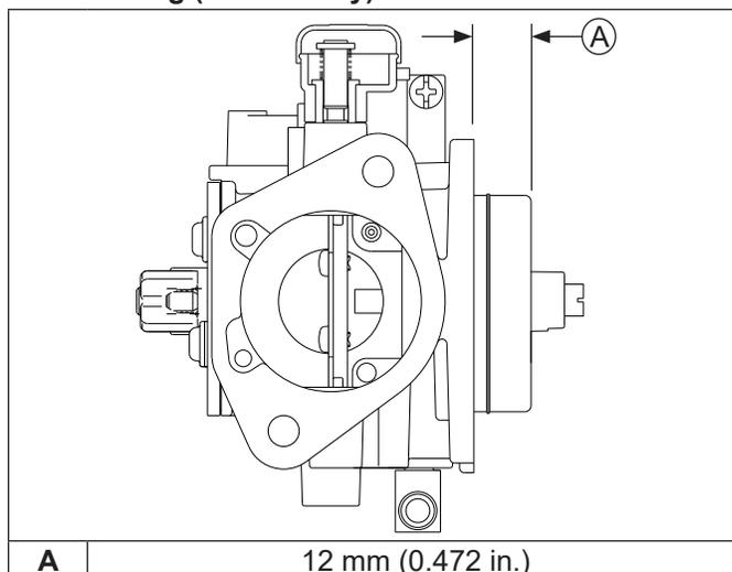
NOTE: Inlet needle center pin is spring loaded. Make sure float assembly rests against fuel inlet needle, without depressing center pin.
