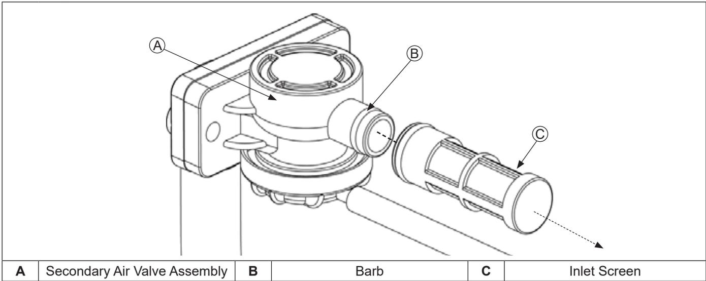
1. Remove inlet screen from secondary air valve assembly by grasping inlet screen at base and gently pulling away from valve assembly.
