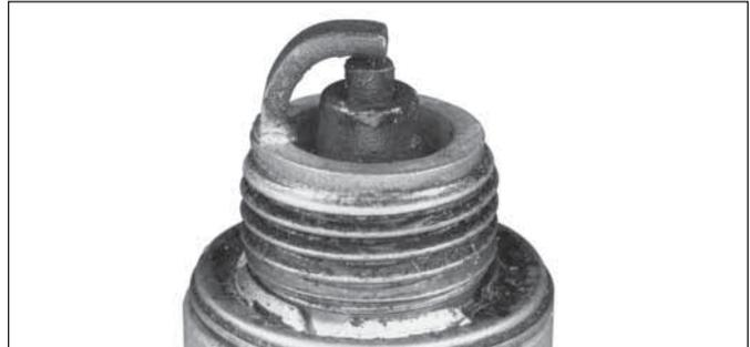
A wet plug is caused by excess fuel or oil in combustion chamber. Excess fuel could be caused by a restricted air cleaner, a fuel mixture problem. Oil in combustion chamber is usually caused by a restricted air cleaner, a breather problem, worn piston rings, or valve guides.
