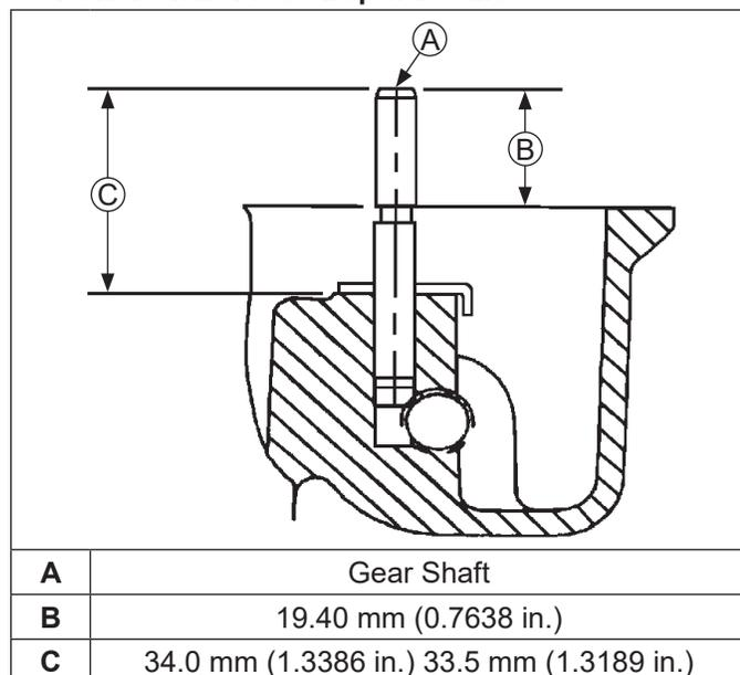
Governor gear assembly is located inside closure plate. If service is required, refer to these procedures.
