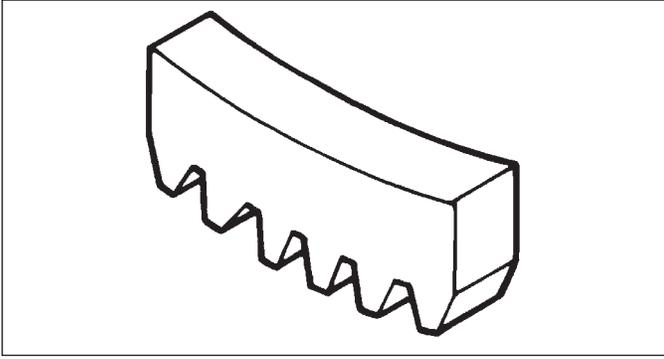
A flywheel holding tool can be made out of an old junk flywheel ring gear and used in place of a strap wrench.
