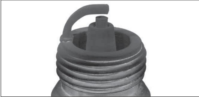
Soft, sooty, black deposits indicate incomplete combustion caused by a restricted air cleaner, over rich fuel mixture, weak ignition, or poor compression.
