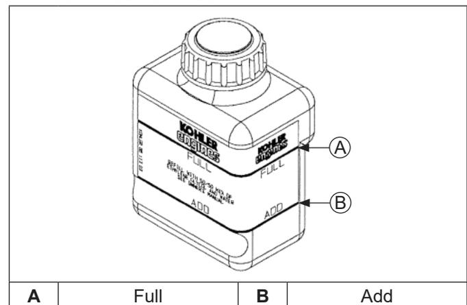
**NOTE:** Do not operate engine without coolant in system. Do not remove radiator cap when hot. Engine coolant is hot and under pressure and can cause severe burns. To prevent engine overheating and damage, do not exceed more than 70% antifreeze in cooling system.
