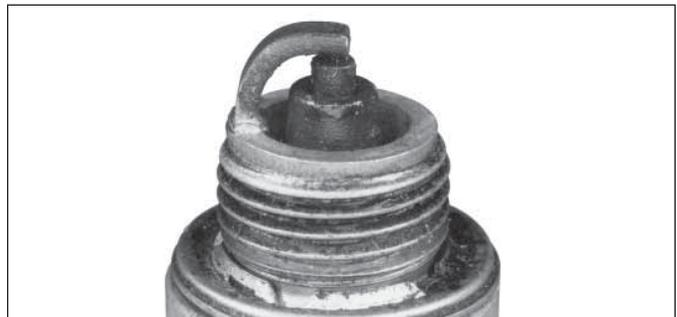
A wet plug is caused by excess fuel or oil in combustion chamber. Excess fuel could be caused by a restricted air cleaner or a fuel mixture problem. Oil in combustion chamber is usually caused by a restricted air cleaner, a breather problem, worn piston rings, or valve guides.
