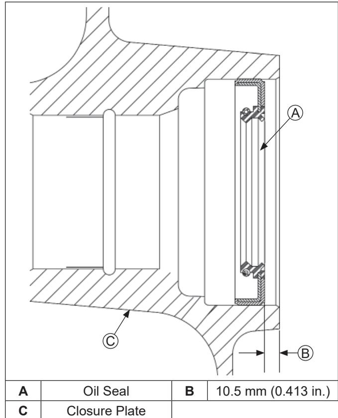
1. Check to make sure that there are no nicks or burrs in crankshaft bore of closure plate.
