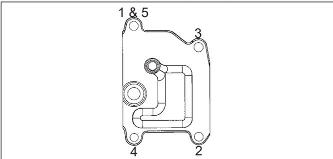
1. Make sure sealing surfaces of crankcase and breather cover are clean and free of all old gasket material. Clean with an aerosol type gasket remover or cleaning solvent. DO NOT scrape surfaces as this can result in leakage.
