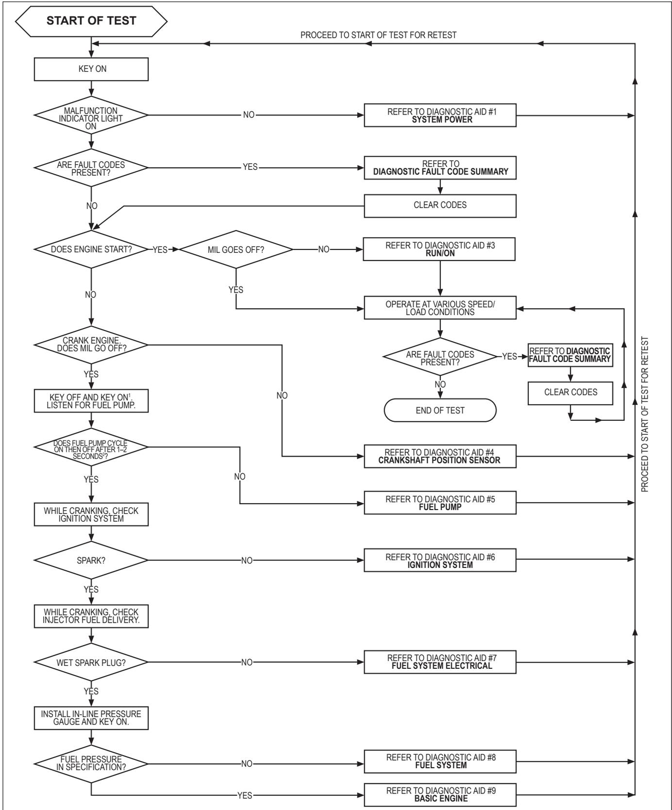
1. After turning key to OFF, wait 10 seconds before turning to ON to allow ECU to go to sleep.
