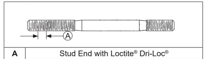
NOTE: Do not reinstall or attempt to reuse any cylinder studs that have been removed. Discard any removed stud(s) and replace with new.
