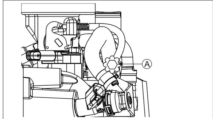
**A** Idle Speed Adjustment Cable
