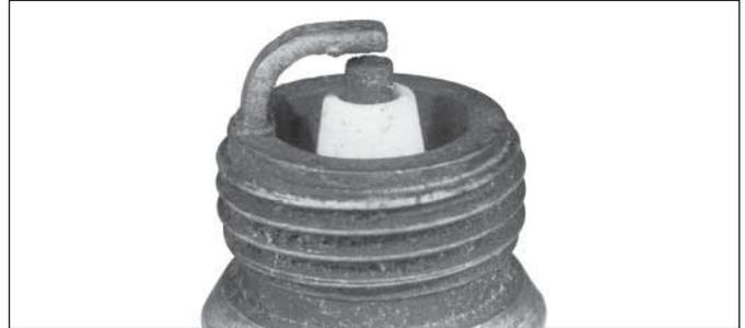
Chalky, white deposits indicate very high combustion temperatures. This condition is usually accompanied by excessive gap erosion. Lean fuel mixture settings, an intake air leak, or incorrect spark timing are normal causes for high combustion temperatures.
