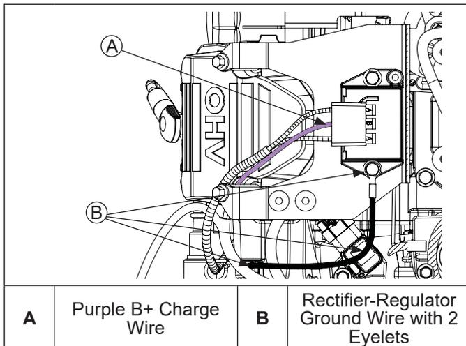
1. With engine off, test and record battery voltage. Voltage should be above 12 volts to proceed. With voltmeter attached to battery, start engine. Set engine speed to high RPM position, battery voltage should increase (for example: 12.6 volts engine off; 13.4 volts engine running). Actual voltage increase will differ depending on state of charge in battery.
