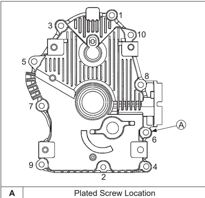
RTV silicone sealant is used as a gasket between closure plate and crankcase. Always use fresh sealant. Using outdated sealant can result in leakage.
