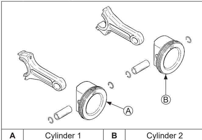
NOTE: Cylinders are numbered on crankcase. Make sure to install piston, connecting rod and end cap into its appropriate cylinder bore, as previously marked at time of disassembly. Do not mix end caps and connecting rods.
