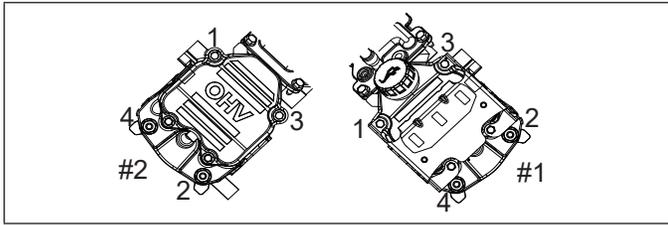
1. Install a new air cleaner adapter gasket onto intake manifold. Make sure that holes align.
