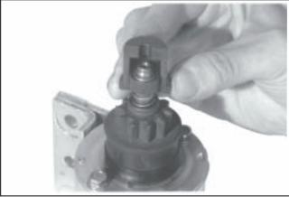
Figure 8-14. Assembling Larger Inner Half Around Spring Retainer.
