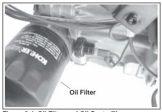
Figure 6-4. Oil Filter and Oil Sentry™.
