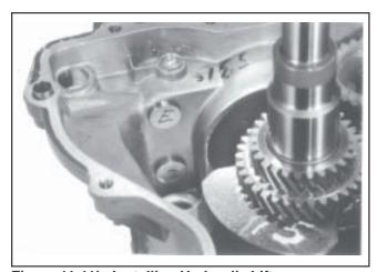
Figure 11-11b. Installing Hydraulic Lifters.
