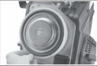
Figure 11-59. Installing Air Cleaner.
