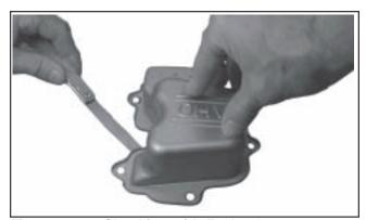
Figure 10-11. Checking with Feeler Gauge.
