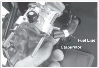
Figure 9-10. Removing Fuel Line From Carburetor.
