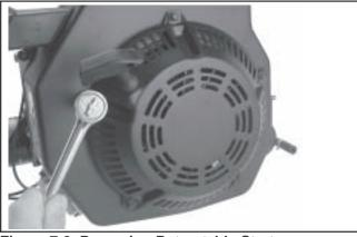
Figure 7-2. Removing Retractable Starter.
