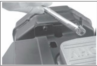
Figure 11-63. Installing Upper Muffler Bracket and Mounting Screws.
