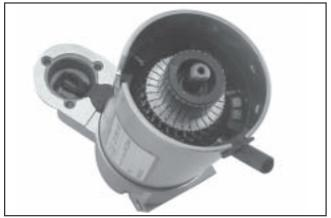
Figure 8-49. Installing Frame and Drain Tube.
