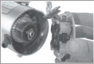
Figure 8-34. Removing Commutator End Plate Assembly.
