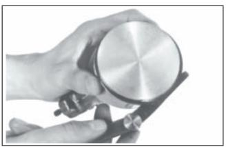
Figure 10-7. Measuring Piston Ring Side Clearance.
