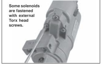
Figure 8-30. Removing Solenoid Screws.
