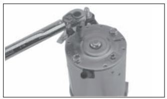
Figure 8-56. Torquing Brush Holder Screws.
