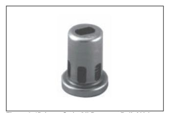
Figure 9-45. Later Style Oil Pressure Relief Valve.
