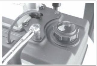
Figure 11-50. Installing Fuel Tank Upper Mounting Screws.
