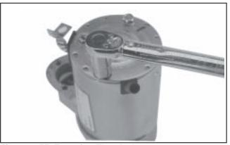
Figure 8-55. Torquing Thru Bolts.
