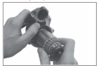
Figure 8-21. Installing Armature.
