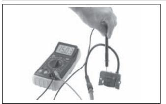
Figure 8-4. Testing Module Secondary.
