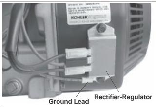
Figure 11-52. Installing Rectifier-Regulator.
