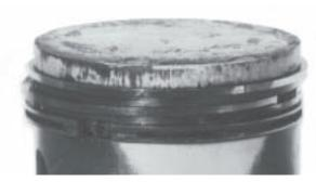
Overheated or Deteriorated Oil
