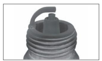
**Carbon Fouled:** Soft, sooty, black deposits indicate incomplete combustion. Incomplete combustion is usually caused by overrich carburetion, weak ignition, or poor compression.
