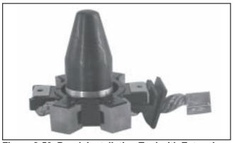
Figure 8-53. Brush Installation Tool with Extension.
