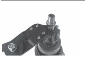
Figure 8-39. Removing Retaining Ring.
