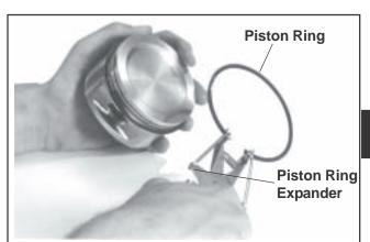
Figure 9-52. Removing Piston Rings.
