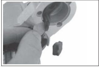
Figure 8-36. Removing Pivot Bushing and Backing Plate.
