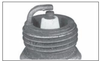
**Chalky White Deposits:** Chalky white colored deposits indicate overheating. This condition is usually accompanied by excessive gap erosion. A clogged grass screen, clogged cooling fins, and lean carburetion are some causes of overheating.
