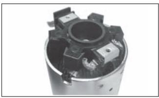
Figure 8-51. Installing Brush Holder Assembly with Supplied Tube.
