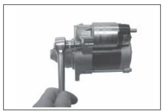
Figure 8-27. Installing Solenoid.
