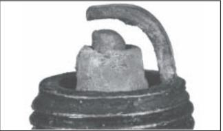
**Worn:** On a worn plug, the center electrode will be rounded and the gap will be eroded .010" or more than the correct gap.
