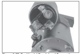
Figure 8-57. Positive (+) Brush Lead Connection.
