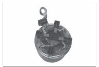
Figure 8-22. Mounting Brush Holder to Frame.
