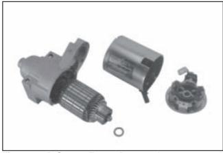
Figure 8-35. Starter Frame Removed.
