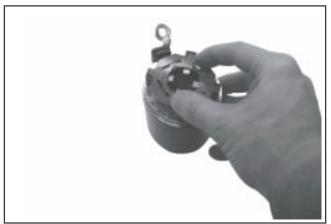
Figure 8-23. Holding Insulator in Place.
