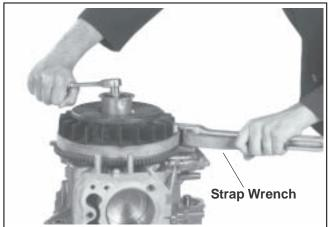
Figure 9-37. Removing Flywheel Retaining Screw and Drive Cup.
