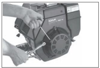
Figure 11-61. Installing Retractable Starter.
