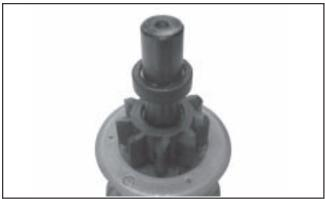
Figure 8-20. Lock Collar around Retaining Ring.
