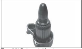
Figure 8-24. Tool on end of Armature.
