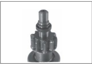
Figure 8-38. Retaining Ring Details.
