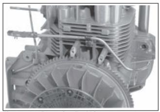
Figure 9-29. Removing Fuel Line.
