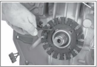
Figure 9-40. Removing Stator.
