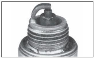
Wet Fouled: A wet plug is caused by excess fuel, or oil in the combustion chamber. Excess fuel could be caused by operating the engine with too much choke. Oil in the combustion chamber is usually caused by worn piston rings or valve guides.
